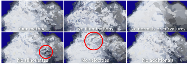
Fig. 13. Ablation study. We compare our full model against versions with individual feature groups removed. Without illumination-related features, the generated colors become noisier; without normals, curvatures, or additional volumetric features, the results appear more monotonous; without the silhouette feature, artifacts emerge (highlighted by the red circle); and without velocity-related features, stroke orientations in vortex regions (red circle) fail to align properly with the flow.
